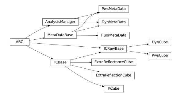
Fig. 1: Abstract base classes define common behavior between the implementations of the various data types making it easy to write software using PWSpy that will work for all available data type implementations.
